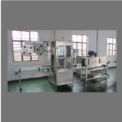
Automatic Double Side Sticker Labeling Machine
