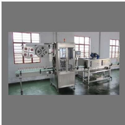
Automatic Shrink Sleeve Labelling Machine (Applicator)
